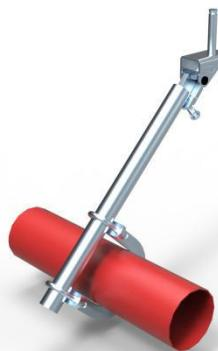
**Function:** Designed for bracing pipe against sway and seismic disturbance. The pipe attachment component of a sway brace system used in conjunction with a UTT Manufacturing structural attachment fitting, and joined together with a bracing pipe element forms a complete sway brace assembly. Sway brace assemblies are intended to be installed in accordance with NFPA 13 and the manufacturer's installation instructions.
